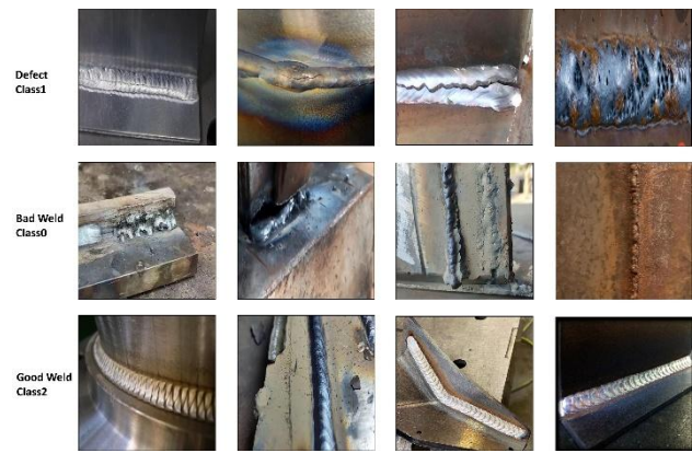
Figure 1. Sample Images from the WD Dataset: Defect, Bad Weld, and Good Weld, Respectively
